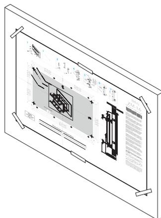
2. Tape appropriate mounting template in place on dash, and ensure cutout lines are level relative to a reference point on dash.
