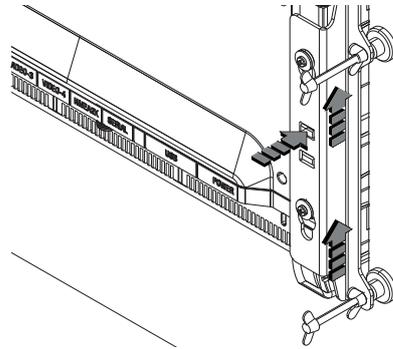
The mounting brackets should be loosened in reverse order to fitting. To remove the brackets, depress the locking tab before sliding brackets upwards.
