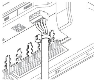
With the cable and plug fitted in place, secure the cable to the retention bracket using a cable tie. Do not secure in such a way that applies strain to the cable, or causes the plug or socket to be bent out of alignment.
