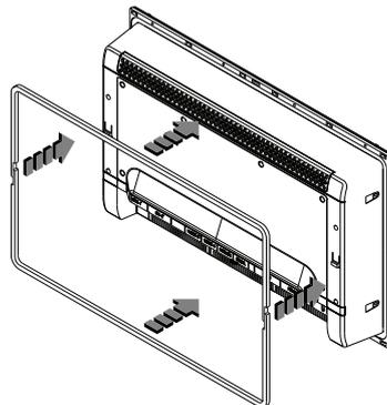
Fit the two lengths of foam gasket in to the rebated channel on the back of the displays mounting flange. Only remove backing paper from the side to be stuck to monitor, and only remove a small amount at a time. Ensure the gasket ends of the two halves overlap and make contact.
