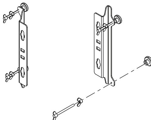
10. Wind wing nut on to wing screw, then wind the wing screw assembly in to bracket till approximately 5 mm of threaded rod protrudes through other side of bracket.
