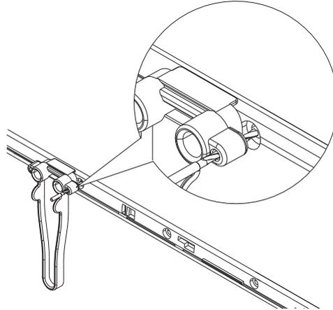
→ **Note:** Before drilling the rest of the pilot holes it is recommended to secure the display with at least one screw to allow for movement in the dash cutout.
